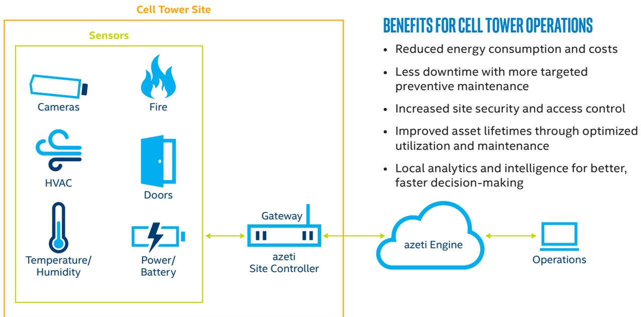
Figure 1. azeti Remote Asset Management Software on Intel-based IoT Gateways.
